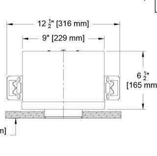
NOTE: This option is intended for use with precise and finished cutouts - usually millwork or wood ceilings. There is no plaster or finish flange.
