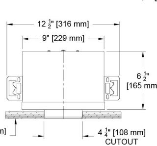
NOTE: This option is intended for use with precise and finished cutouts. There is no plaster or finish flange.
